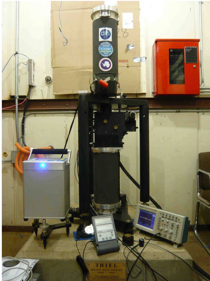
Figure 2.3: FG5 #228 installed over Thiel-1 benchmark. Scintrex CG-5 on the left on the pillar.
