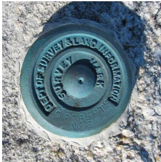
Figure 4.2: Location of the LINZ CRN2 benchmark (bottom left-hand corner of the top image) near the tide gauge and GPS antenna (top).
