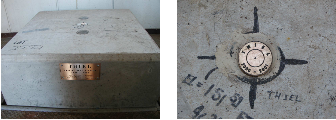
Figure 2.2: Concrete pier and Thiel-1 benchmark inside Thiel observatory (building 146).
