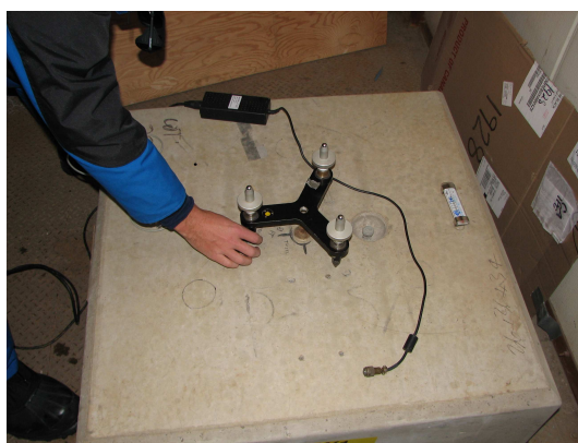
Figure 2.5: Tripod of Scintrex-CG5 over Thiel-1 benchmark.
