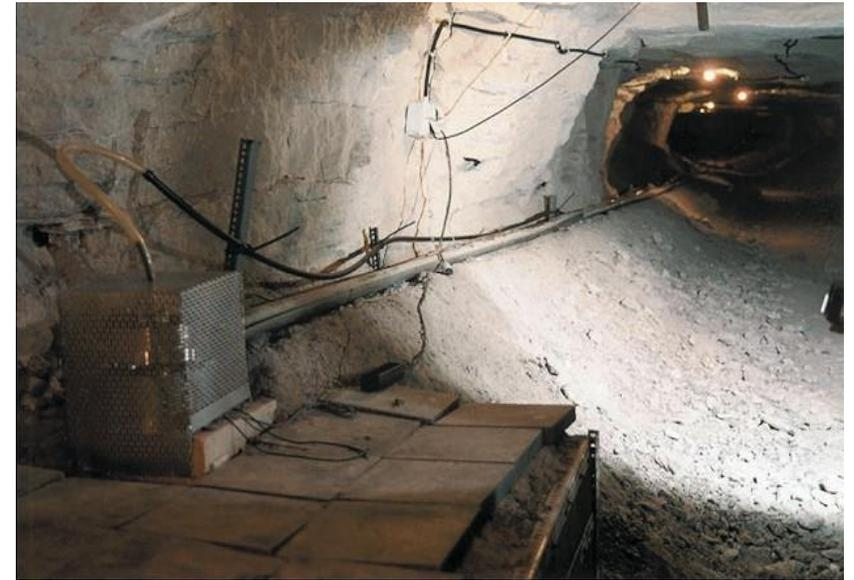
Water tube tiltmeter at the Underground Laboratory of Geodynamics (N. d'Oreye)
