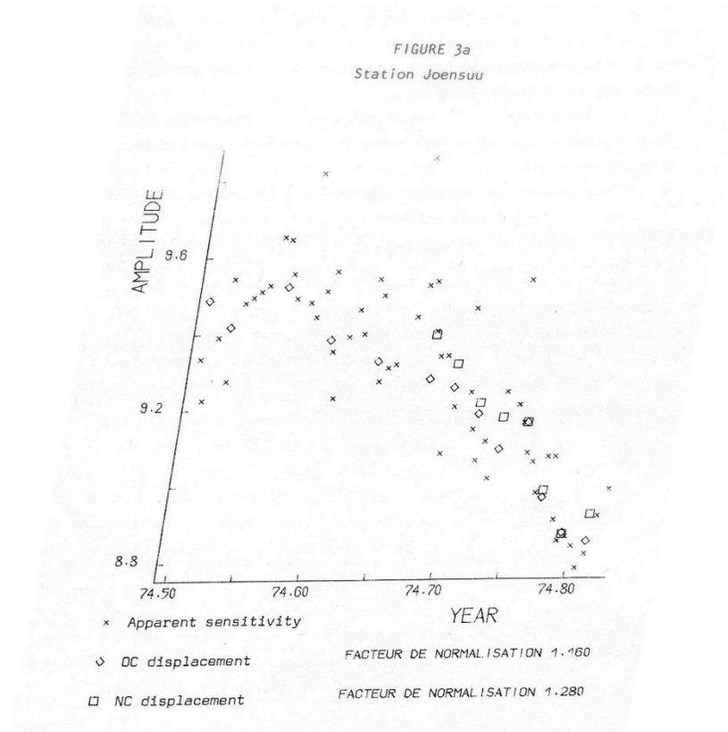
Variation of sensitivity of an astaticized gravimeter
