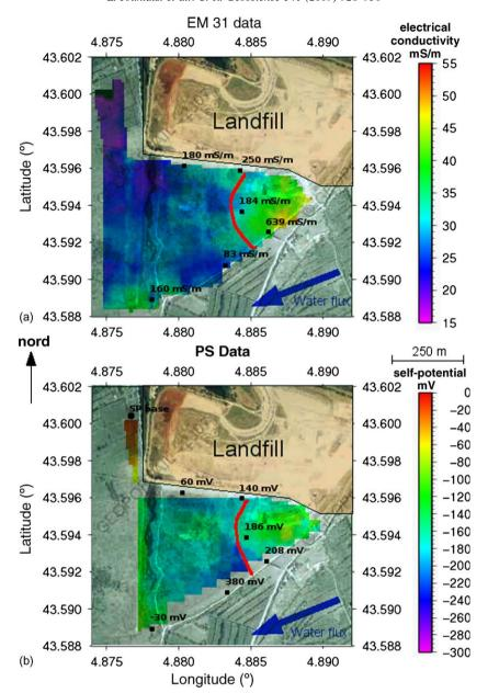
Fig. 2. Observations performed downstream the Entressen landfill: (a): electrical conductivity map (in millisiemens per metre) and water conductivity measured in boreholes (black points); (b): SP map (in millivolts) with the redox potential (Eh) values measured in boreholes (black points). Water conductivity and redox potential measured upstream the landfill are respectively 70 mS/m and 150 mV.
