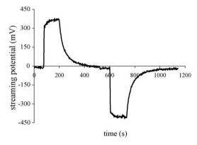
Fig. 1. Example of measured streaming potential  $\Delta V$  when the applied driving pore pressure is 0.1 MPa in one way (positive signal) and in the reverse way (negative signal) within a sandstone sample. Water resistivity is  $720 \, \varsigma \, m$ , and permeability is  $6.5 \times 10^{-14} \, m^2$ .
