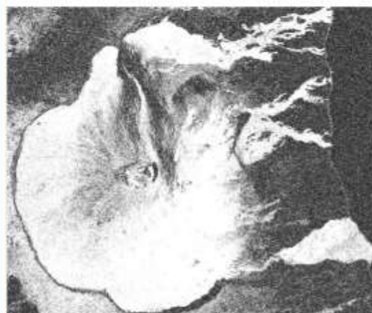
Coherence image after the eruption on April 03, 2018 (between two images acquired on March 23 and April 04, 2018)
