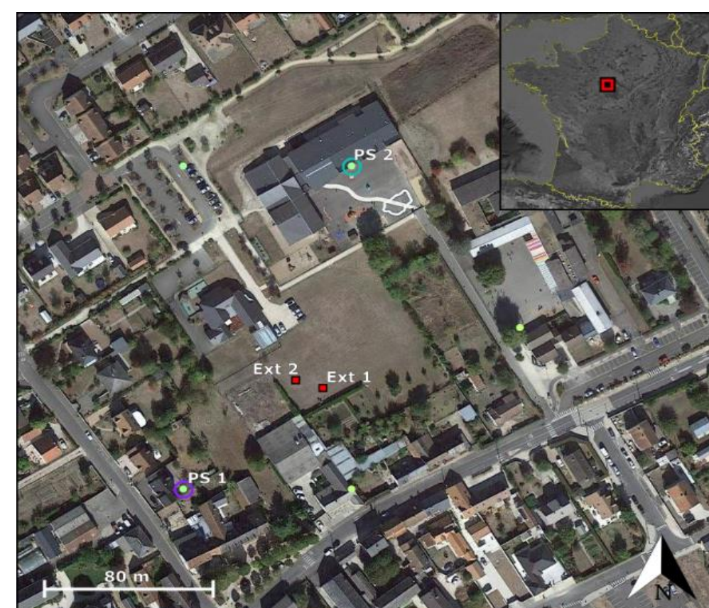
Ext 1 and 2 extensometer location map and SqueeSARTM PS 1 and 2 vertical points in the city of Chaingy
