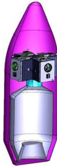
Vega-C rocket fairing accommodating 4 CO3D satellites
