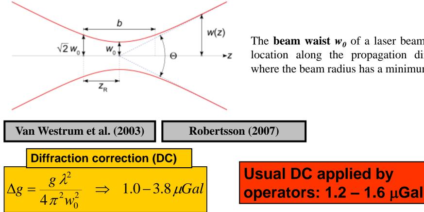
The **beam waist**  $w_0$  of a laser beam is the location along the propagation direction where the beam radius has a minimum.
