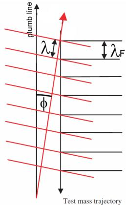
If the laser is not aligned along the plumb line, the test mass falls distance of  $\lambda_F = \lambda / \cos \varphi$  (longer than the measured distance  $\lambda$ ). Therefore, the **measured gravity**  $g_m$  becomes **lower** than the "real" g.
