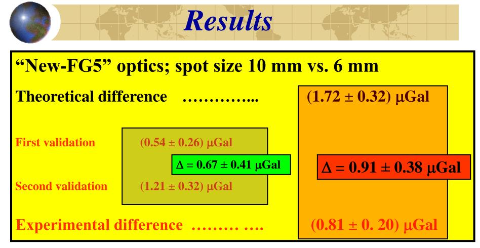
The experiment showed on the **measurable difference** of  $0.8 \pm 0.2 \mu$ Gal for a typical **spot sizes of** FG5s ranging from 6 mm to 10 mm. However, the theoretical difference should reach  $1.7 \pm 0.3 \mu$ Gal (for an ideal Gaussian beam).
