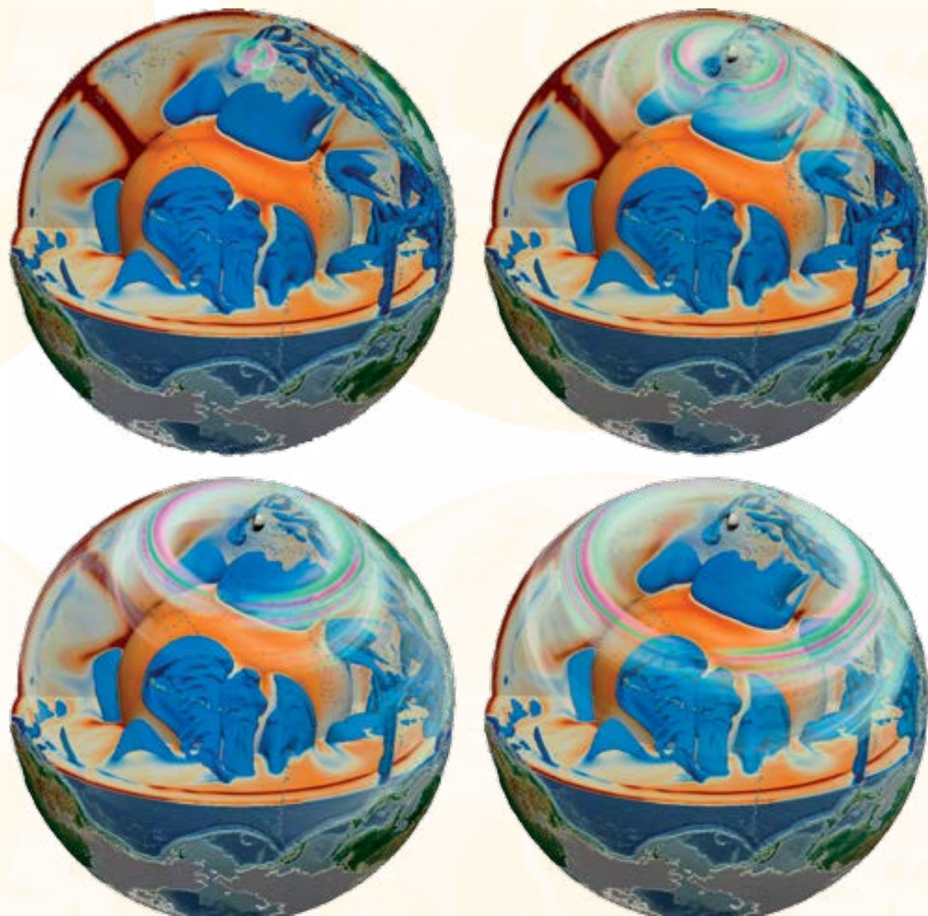
Figure 1: Snapshots of the three-dimensional wavefield in one of our geodynamic models. 3-D global wave propagation was simulated for an earthquake in the Fiji Islands region using a spectral element technique. The wavefield is depicted by green and magenta colours together with the shear wave velocity variations in the model, for which vertical cross-sections and iso-surfaces are shown on a blue to brownish colour scale ranging from -2 to 2 per cent. Surface topography is also shown for parts of the globe for geographic reference [1]
